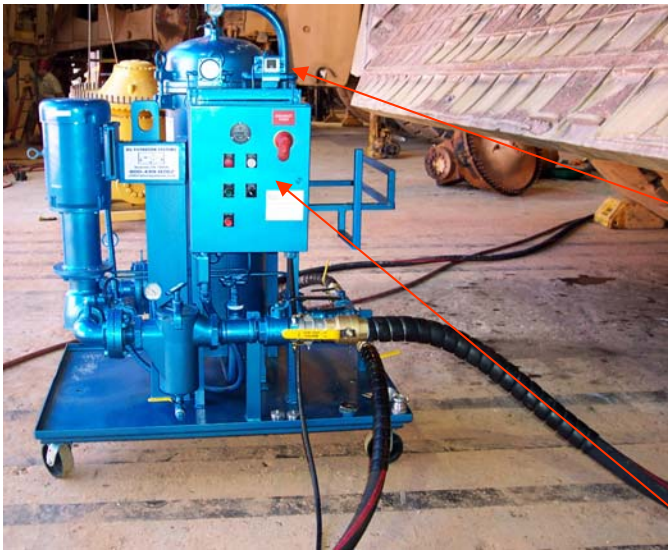
40 GPM Filtration System
