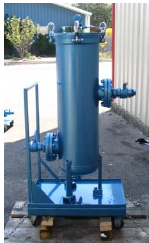
High Flow Particulate Removal Filter Vessel
