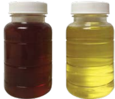
Before Filtration ISO 22/21/19 MPC* Value = 38
